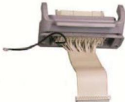
6. Reconnect the encoder cables to EXE 932: Y to X3; Z to X2; X to X1.
